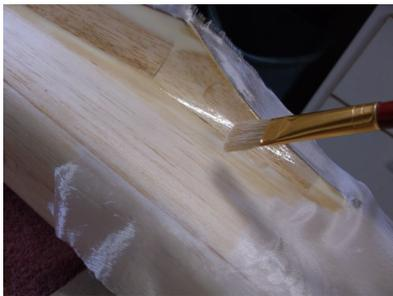
**Brushing through lite weight cloth with resin removing wrinkles as you go.**
