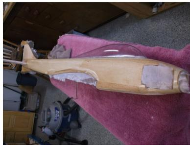
**epoxy curing , securing glass cloth**
