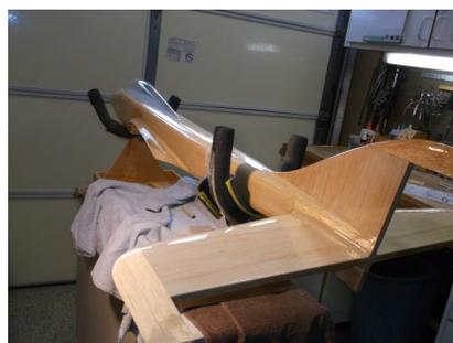
**The 2nd coat of resin After the initial glass cloth Application coat. The sanding Is minimal until the last coat Of resin and then you really Have to go to work.**
