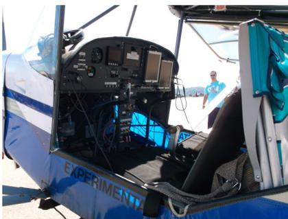
This homebuilt Ultra-lite was flown from California to Oshkosh for the EAA Fly-in . The motor is water cooled and the motor uses regular gas and has a rescue parachute attached to the airframe. By the way the owner is a very gutsy interesting Lady , Rene .
